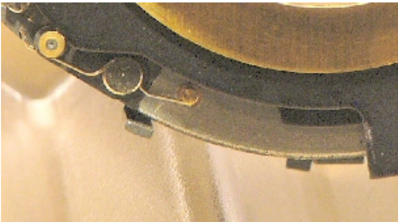
PIC 7: Diaphragm roller (lens cocked)
